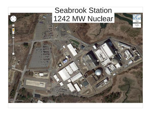
And this is the smudge blown up to a useful size. The original plans were for two plants, only the one on the right was completed. The round buildings are the reactor containment structures, the turbines are adjacent, up and to the left.
