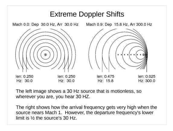
Neither of these apply to passing helicopters. A hovering 'copter has no Doppler shift, nor can a helicopter fly at the speed of sound (the forward moving blade tip would be faster than the speed of sound) and the other side would have very little lift – and zero lift when the first side was at Mach 2!
