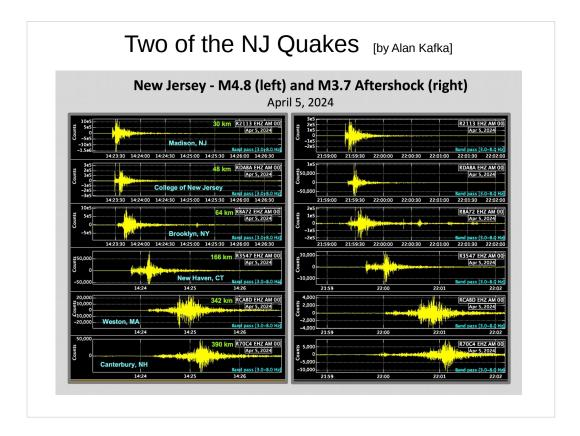
This shows the main quake on the left and the biggest aftershock on the right as recorded by five Raspberry shakes. While the placement of the seismographs has a lot to do with the strength seen at the stations, the "counts" (vertical speed) is as strong in Brooklyn as it is nearest the epicenter.
