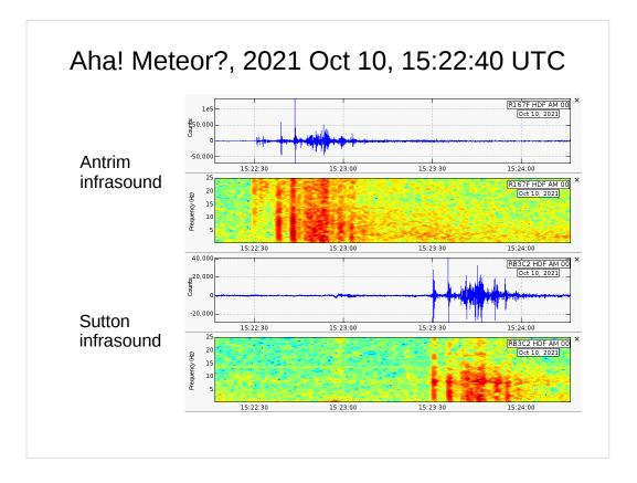
I soon found similar recordings at Antrim, but louder and earlier and with higher frequencies still present. The spacing between booms was nearly identical. This supported a single location for the source and that for a meteor the sounds were from the breakup and not sonic booms.
