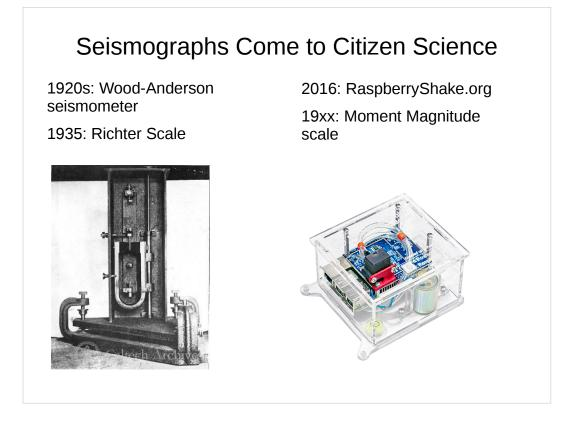
The well known "Richter Scale" is tied to this particular seismometer. It was replaced with the Moment Magnitude Scale, a measure of energy released in an earthquake.
