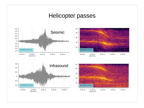
Of all the aircraft in the sky, helicopters and the Doppler effect due to their rotor stand out exceedingly well. It appears that the pulses couple into the ground surprisingly well, especially (and not surprisingly) when the spherical wavefronts are directly over the ground.
