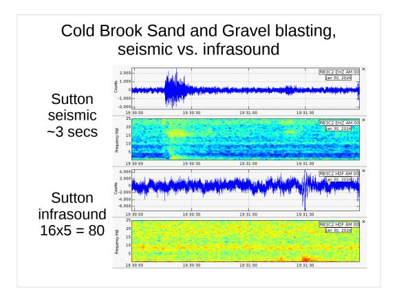
The Canterbury site is a Shake, but not Boom, and doesn't record sound, my Shake and Boom records both. Sound takes about five seconds to travel one mile, so it should (and does) take about eighty seconds to reach me. Very cool!
